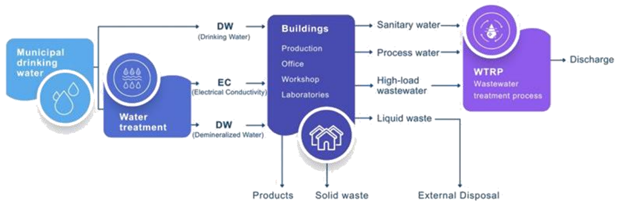
Figure 3: Physical system boundaries and water, wastewater, and waste flow structure within a pharmaceutical production site as represented in the ENVIROMED registry.
